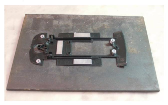
Put the iron sheet with the clamped chassis in the glass pan.
