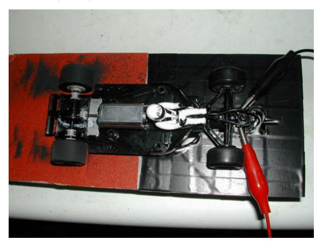
With the electrical leads from my power supply connected to the car's guide flag wipers/braid, with the power "on", while the motor is running I gently lower the rear of the chassis onto the test block sandpaper.
