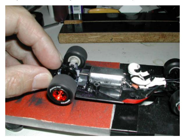
Take your time with the sanding and monitor the motor's temperature.
