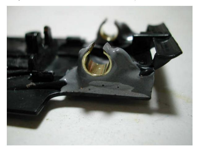
The slot cut into the tubing should be just wide enough for the axle to slip through.
