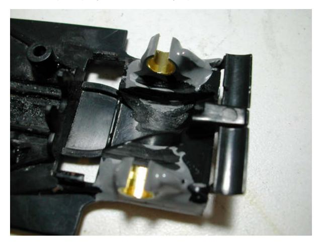
It may take a couple applications of JB Weld to get it "built up" around the tubing. The JB Weld wants to run a bit before it hardens up.
