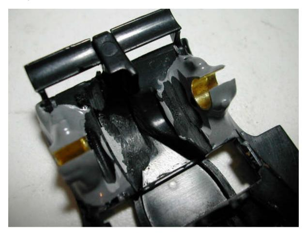
Below are photos of the finished repair which allows the use of standard 3/32 oilites, and a 3/32 axle assembly (standard slot car parts for commercial track type slot cars).
