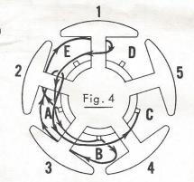
& 3 with the SAME NUMBER OF TURNS as segments 1 & 2. After segments 2 & 3 are wound, solder the wire to point C.
