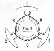
PING.) Continue winding segment 2 in a clockwise direction. Wind segment 2 with the SAME NUMBER OF TURNS as segment 1.
